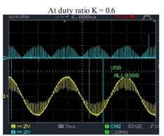
Fig. 7 Blue waveform shows voltage across switch (Vsw) Yellow waveform shows voltage across load (V0) Vsw = V0 = 200 volts/division Time T = 5 millisecond/division
