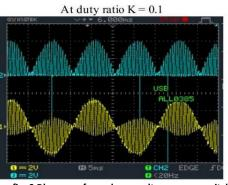
fig. 9 Blue waveform shows voltage across switch (Vsw) Yellow waveform shows voltage across load (V0) Vsw = V0 = 200 volts/division Time T = 5 millisecond/division
