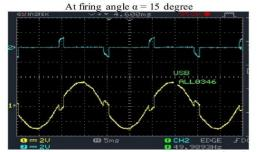
Fig.2 Blue waveform shows voltage across switch (Vsw) Yellow waveform shows voltage across load (V0) Vsw = V0 = 200 volts/division Time T = 5 millisecond/division
