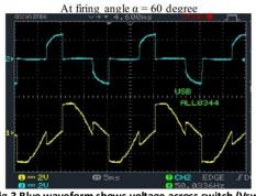
Fig.3 Blue waveform shows voltage across switch (Vsw) Yellow waveform shows voltage across load (V0)
