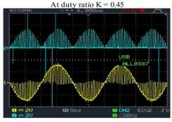
Blue waveform shows voltage across switch (Vsw) Yellow waveform shows voltage across load (V0) Vsw = V0 = 200 volts/division Time T = 5 millisecond/division
